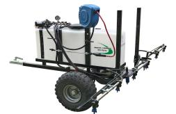
Mini-Spray Trailed 125 litre with 2.5m 6-nozzle 3-section folding boom and retracting hose reel with hand lance
